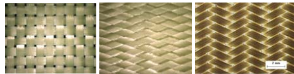
Figure 1. from left to right: a) plain weave, b) trellised biaxial and c) standard braid triaxial fabrics
